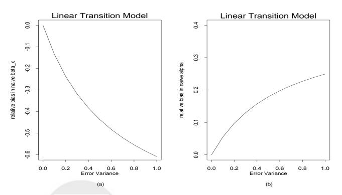
Figure 1: Asymptotic relative biases in naive estimators of  $\beta_x$  and  $\alpha$  by ignoring measurement error in the first order linear transition measurement error model for Gaussian outcomes. The true parameter values are  $\beta_0 = -1$ ,  $\beta_x = 1$ ,  $\alpha = 0.5$ ,  $\sigma^2 = 1$ , and  $\gamma_0 = 0.4$ ,  $\gamma_x = 0.6$ ,  $\sigma_x^2 = 0.5$ . The two plots correspond to (a) the relative bias in  $\beta_{x,naive}$ ; (b) the relative bias in  $\alpha_{naive}$ .
