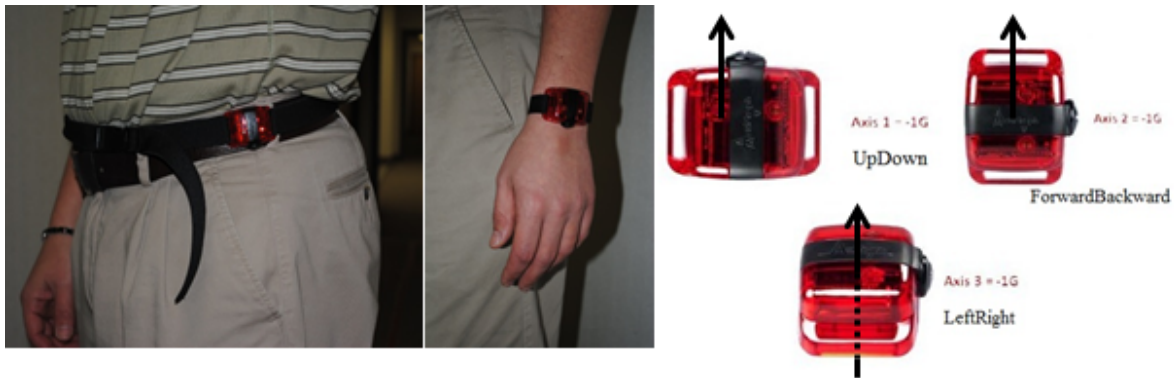
Figure 1: Accelerometer placement on the body. The left and middle panels present how an accelerometer was attached to hip and wrist, respectively. Accelerometers have the same orientation. The right panel illustrates how the three axes of signals in the output are denoted.
